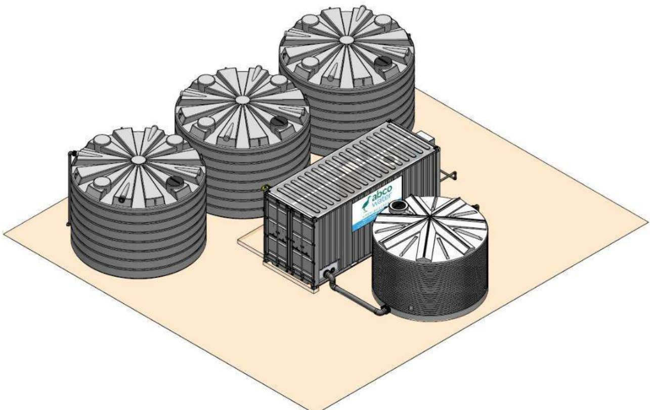
ABCO containerised RO plant
