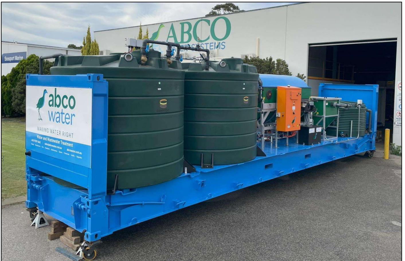
ABCO 15 m 3 /day skid mounted RBC plant
