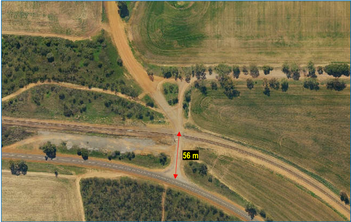
Figure 12: Approach Sight Distance Measurement
