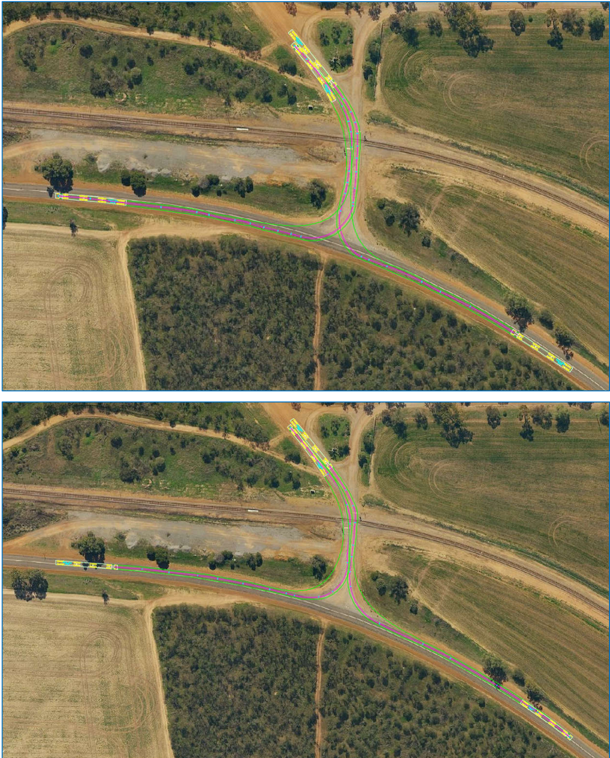
Figure 20: Intersection 2 Swept path Analysis
