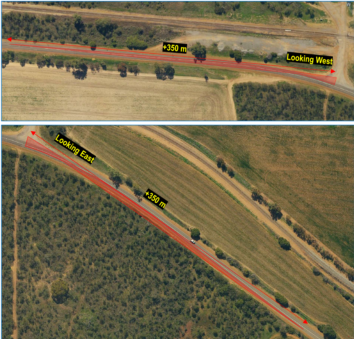
Figure 9: Sight Distance Measurement at Intersection 2
