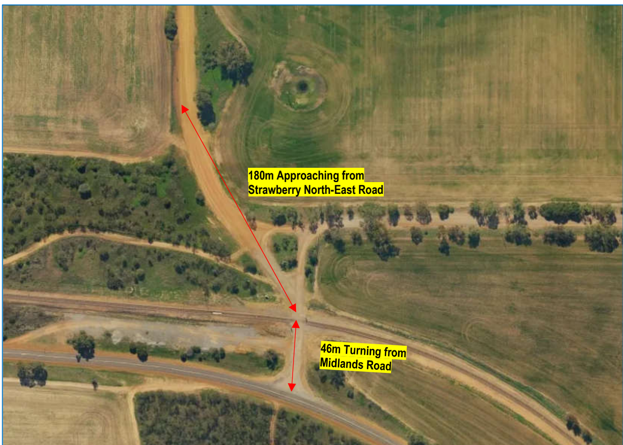
Figure 21: Approach Sight Distance Measurement
